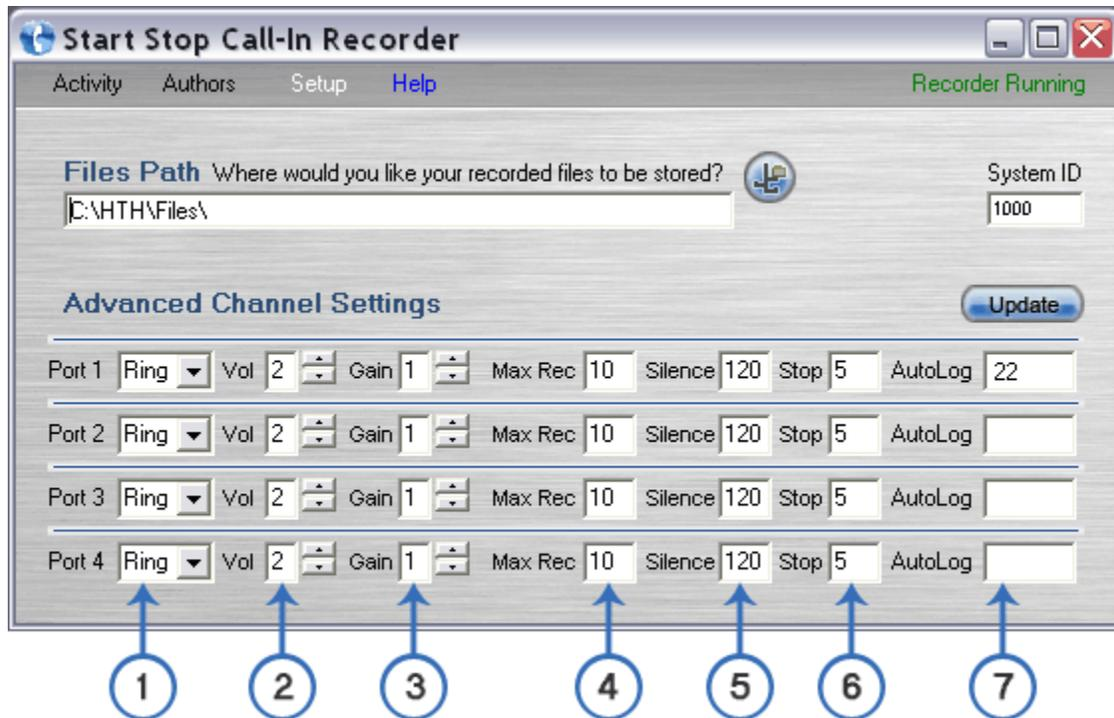
**1. Loop/Ring.** Set to **Ring** if a telephone or DID line is connected to that channel. Set to **Loop** only if a direct-wired telephony station is connected to that channel.
